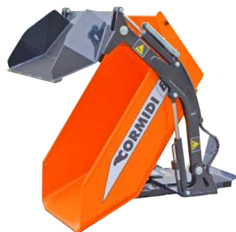
dumper skip + self loading with swivel bucket
