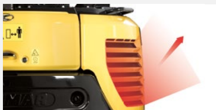
Engine air cooling evacuation facing up (protection of people and the surrounding plants)
