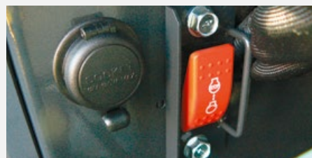
Electric engine stop (emergency stop)
